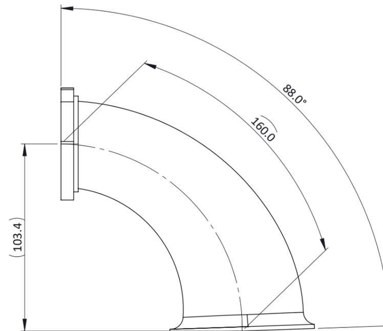
ALUMINIUM CAST AIR HORN WITH A Ø42MM BORE AND 160mm EFFECTIVE LENGTH WITH A 88° CURVE.
