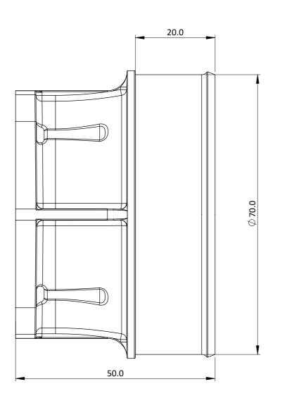
A small lightweight cast aluminium spigot to fit an individual throttle body 52-54mm bore. Ideal for a 70mm silicone hose.
