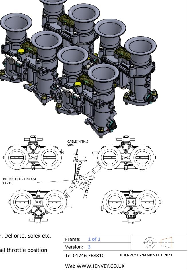
The Heritage body is designed with major dimensions identical to twin vertical carburettors from Weber, Dellorto, Solex etc. The fuel rail is integrated within the body lid, supplied with Bosch EV14 730cc/min injectors. The body comes with 'O' rings on the outlet, idle bypass adjustment, 60mm long air-horns and an internal throttle position sensor.
