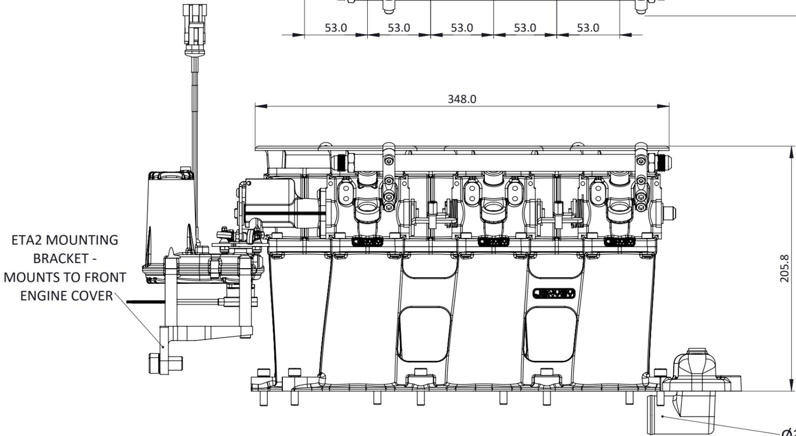
THE JENVEY, FORD 3.7L CYCLONE DOWNDRAFT KIT INCLUDES MANIFOLDS, Ø51MM SF THROTTLE BODIES, 19MM AIRHORNS, FUEL RAILS + MOUNTS, \*WATER MANIFOLD, JENVEY ETA2, MOUNTING BRACKET & LINKAGE, & TP3 THROTTLE POSITION SENSOR.
