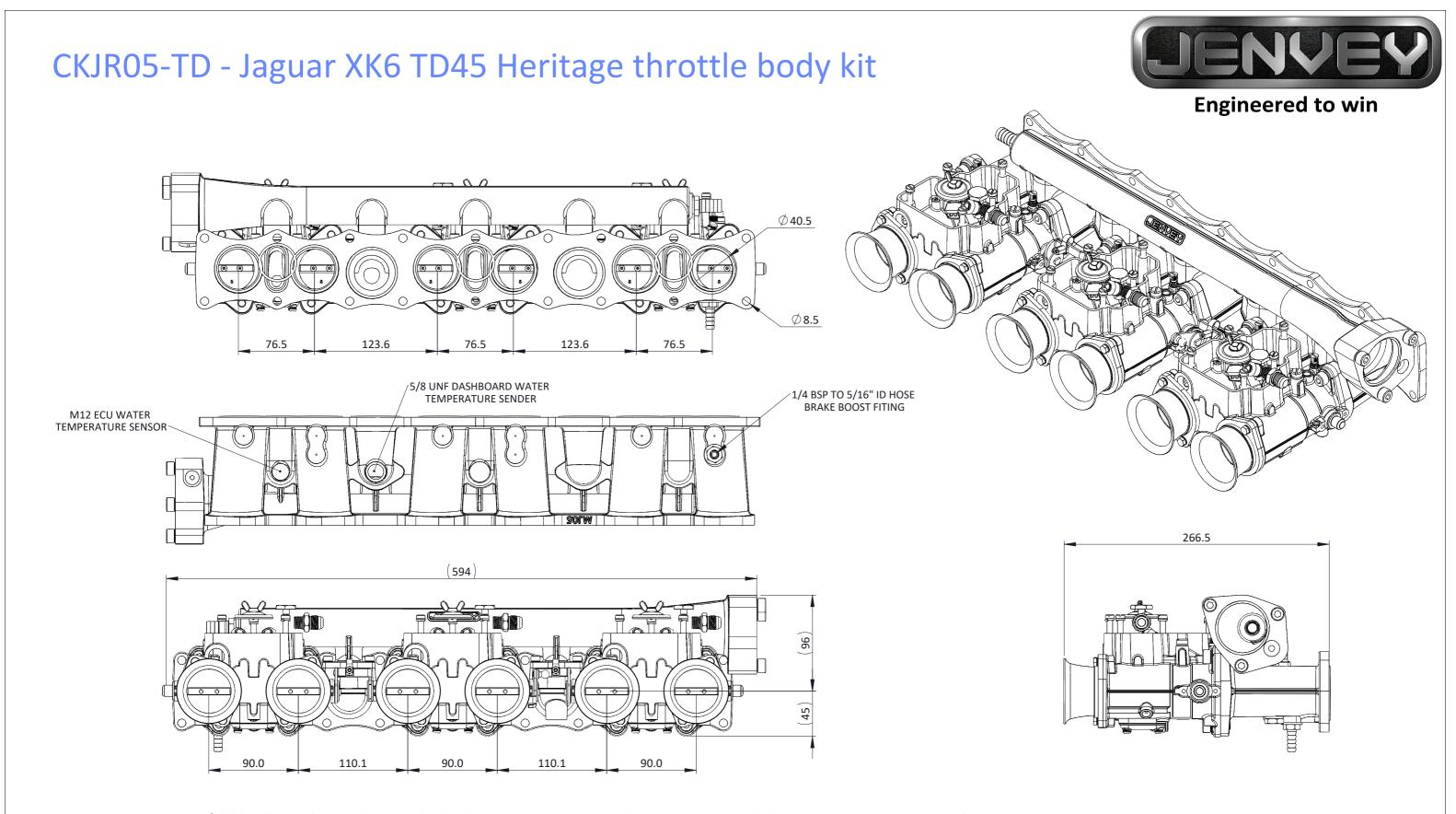
The Jenvey Jaguar XK6 manifold has been designed to suit both the E-Type Series 1 3.8L & 4.2L engines and the Series 2 4.2L engine, With inlet flanges to suit Jenvey DCOE Heritage and standard throttle bodies.
