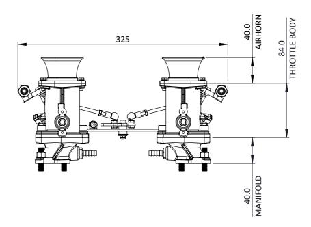
AN INDIVIDUAL THROTTLE BODY KIT FOR THE JAGUAR V12 WHICH CONTAINS A SET OF SIX INLET MANIFOLDS, SIX 40mm TF THROTTLE BODIES AND 40mm LONG HERITAGE AIRHORNS.
