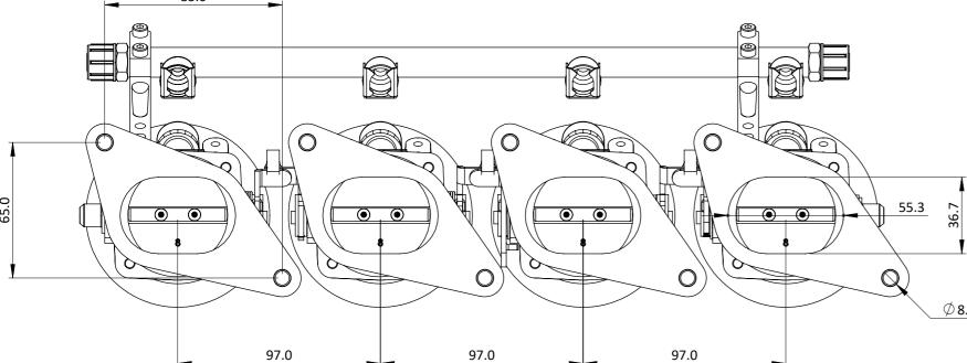
High Port SR20VE - Will not fit the DET version Four 48mm taper throttle bodies, fuel rail with mountings and 90mm long airhorns. This engine was used in the Primera and other Nissan's Bottom flange is the same as SR20DE - will work with a SR20DE block and SR20VE head
