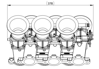
A KIT FOR THE NISSAN VQ SERIES ENGINE WHICH INCLUDES A PAIR OF MANIFOLDS, SIX 51mm SF51 TAPERED BODIES, LINKAGE, FUEL RAILS WITH DASH 6 ENDS AND SIX AHT51X83 STRAIGHT AIRHORNS. (DOES NOT INCLUDE INJECTORS) NOTE, THIS KIT DOES NOT FIT UNDER THE 350Z BONNET. SEE CKNN02C FOR THE 350Z KIT. THE ENGINE IS USED BY INFINITI IN SEVERAL MODELS IN THE US AND THE 350Z IN THE UK AS WELL AS CERTAIN RENAULTS. MADE TO ORDER.
