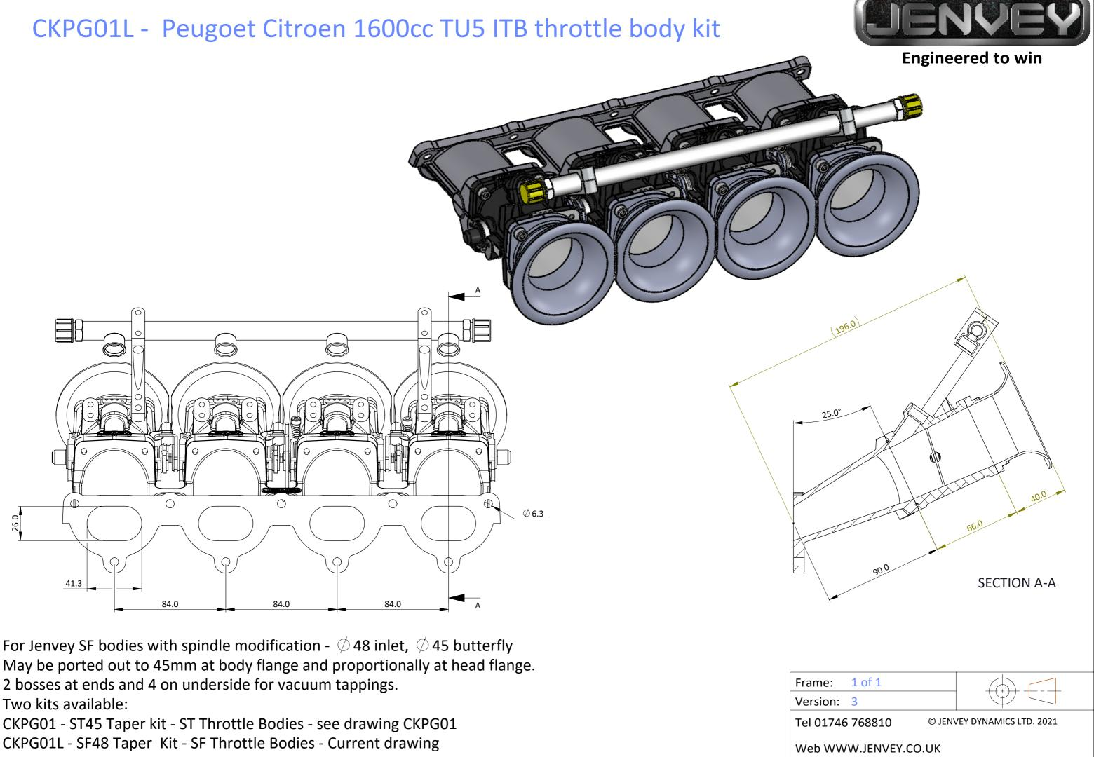
2 bosses at ends and 4 on underside for vacuum tappings.
