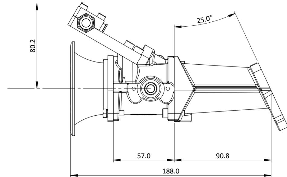
The Jenvey Dynamics tapered CKPG04 kit promises enhanced performance and better throttle control for the TU5JP4 & TU5JP4s engine as found in the VTS, VTR & GT models. This kit contains, an inlet manifold, four ST45 tapered throttle bodies (42mm butterfly), fuel rail, fuel rail mounts and 40mm long airhorns. Where space is available 90mm airhorns further improve performance.
