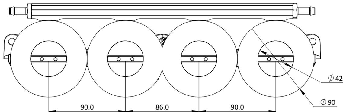
Rover Individual Throttle Body (ITB) kit for fuel injecting your Rover K series engine which contains a linked pair of Ø42mm throttle bodies which attach directly to the cylinder head and four 90mm long air horns. This engine was used in Rover Metro, 200, MGF, Lotus Elise, Caterham and many kit cars. Made to order.
