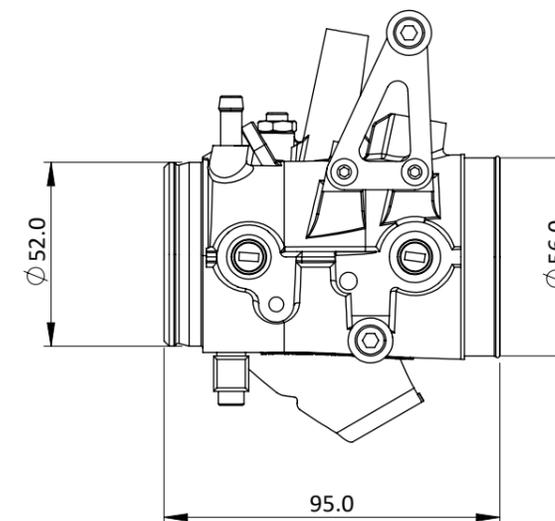
A KIT FOR THE GEN 2 (POST 2008) SUZUKI HAYABUSA ENGINE - USES TWO, TWIN Ø48 BUTTERFLY THROTTLE BODIES WHILST RETAINING THE USAGE OF THE STANDARD FUEL RAIL, INJECTORS, FRONT SPINDLE TPS, REAR SPINDLE ETA MOTOR & TPS, MOUNTING RUBBERS, AIRHORN RUBBERS AND CABLE TRAVEL DISTANCE.
