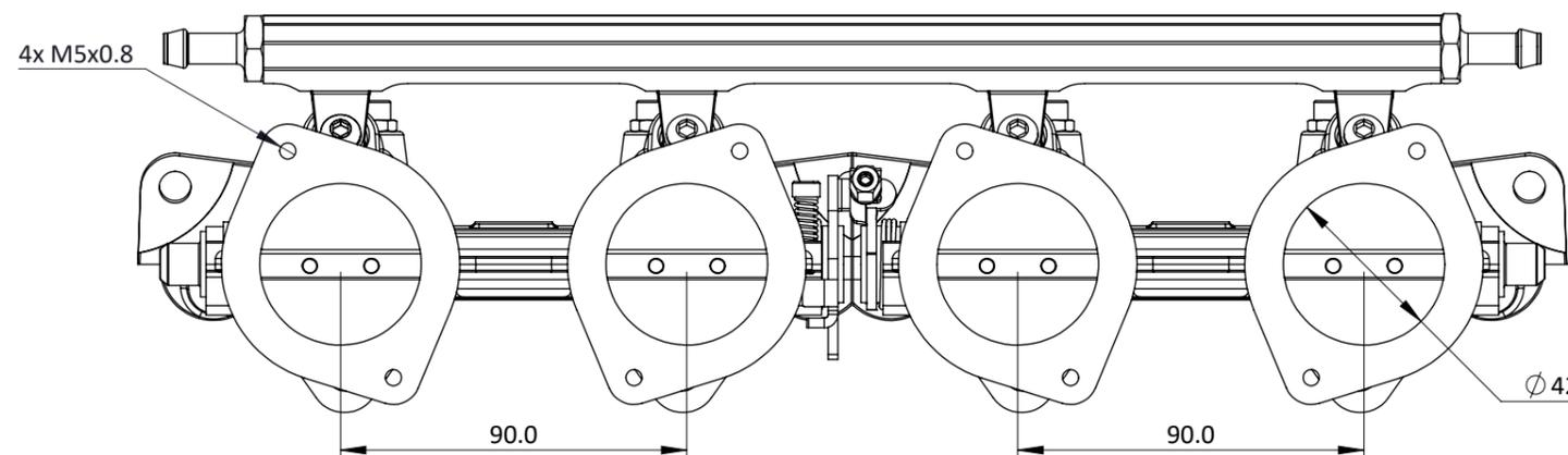
Rover Individual Throttle Body (ITB) kit for fuel injecting your Rover K series engine which contains a linked pair of Ø42mm throttle bodies which attach directly to the cylinder head, fuel rail optional. This engine was used in Rover Metro, 200, MGF, Lotus Elise, Caterham and many kit cars. Made to order.
