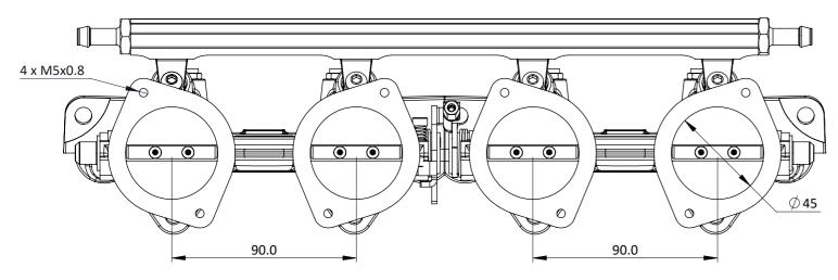
Rover Individual Throttle Body (ITB) kit for fuel injecting your Rover K series VVC engine which contains a linked pair of Ø45mm throttle bodies which attach directly to the cylinder head, fuel rail optional. This engine was used in Rover 200, MGF, Lotus Elise, Caterham and many kit cars. Made to order.
