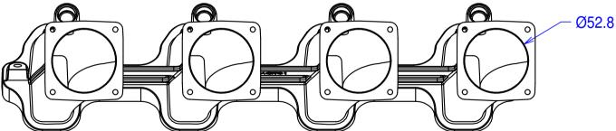
Flanges for Jenvey SFD throttle bodies. Sufficient metal to allow for port machining, including 'Cathedral' shape. 'O' ring seal to cylinder head.
