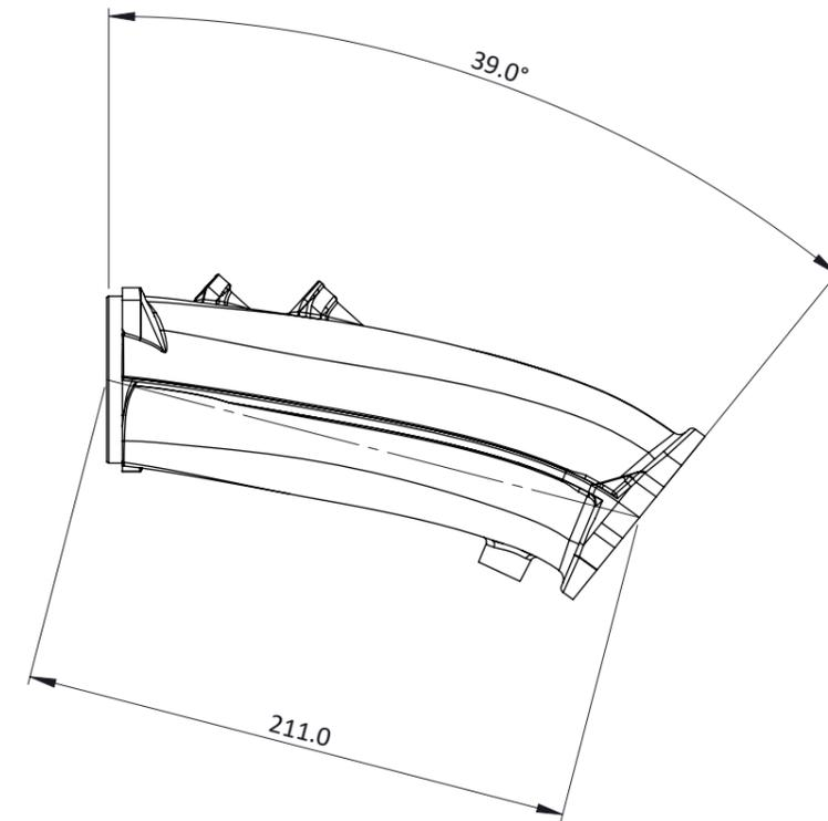
FLANGES FOR JENVEY SSD SPIGOT BODIES, HEAD FLANGE MAY BE PORTED TO SUIT CYLINDER HEAD, BUT NOT THE THROTTLE BODY FLANGE.
