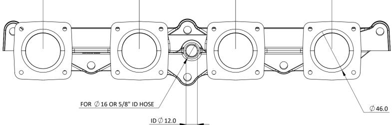
FORD PINTO 2.0 MANIFOLD, WITH FLANGES TO SUIT JENVEY SF INDIVIDUAL THROTTLE BODIES. ADDITIONAL MATERIAL AROUND OUTLET PORT, TO ALLOW FOR MATCHING TO PORTED CYLINDER HEADS UNDRILLED BOSSES ON UNDERSIDE OF MANIFOLD, FOR IDLE AIR/ VACUUM TAKE-OFFS ETC.
