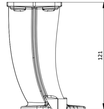
A downdraft style inlet manifold for the Ford Cyclone V6. This manifold is for 6 individual SF throttle bodies 50mm parallel. Includes separate water housing.
