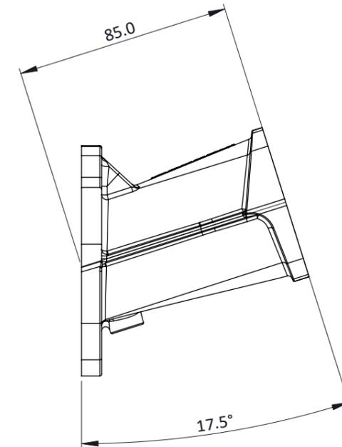
MAY BE PORTED OUT TO 52MM AT INLET FLANGE AND PROPORTIONALLY AT HEAD FLANGE.
