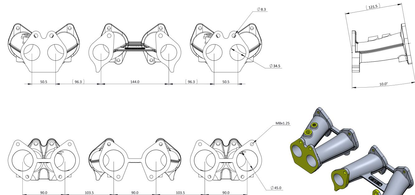
NISSAN DATSUN MANIFOLD SET FOR 240Z, 260Z, 280Z, 280ZX. THIS SET OF MANIFOLDS FITS TO THE DATSUN L-SERIES 6 CYLINDER ENGINES (L24, L26 & L28) THE MANIFOLD HAS A 45mm INLET (WHICH CAN BE PORTED UP TO 48mm) AND 34.5mm OUTLET IT CAN BE USED WITH ANY DCOE STYLE FLANGE THROTTLE BODY.
