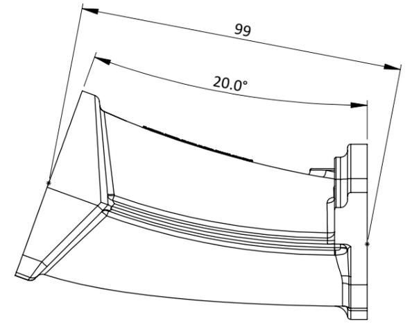
Inlet manifold for ST throttle bodies to fit a Toyota Yaris 1.5 litre. Ø45mm inlet, can be ported to head. Includes extra undrilled bosses on the side for idle air / vacuum take off / etc.
