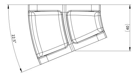
A CAST ALUMINIUM SPACER THAT CURVES THROUGH AN ANGLE OF 22.5 DEGREES. 42MM BORE SKU: SCS42\_22.5 45MM BORE SKU: SCS45\_22.5 48MM BORE SKU: SCS48\_22.5
