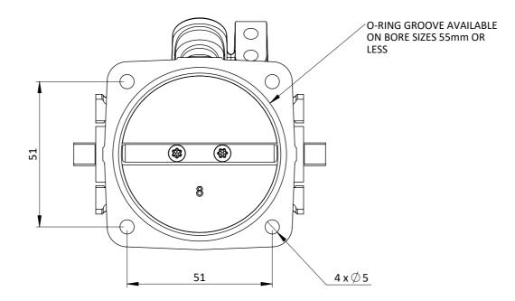
THE SDS BODY FITS THE SAME FLANGES AS THE SFD RANGE AND IS ONLY AVAILABLE WITH AN INJECTOR POCKET. IT IS AN EXTREMELY COMPACT BODY ALLOWING VERY LONG AIR HORNS TO BE USED WITHIN A GIVEN SYSTEM LENGTH.
