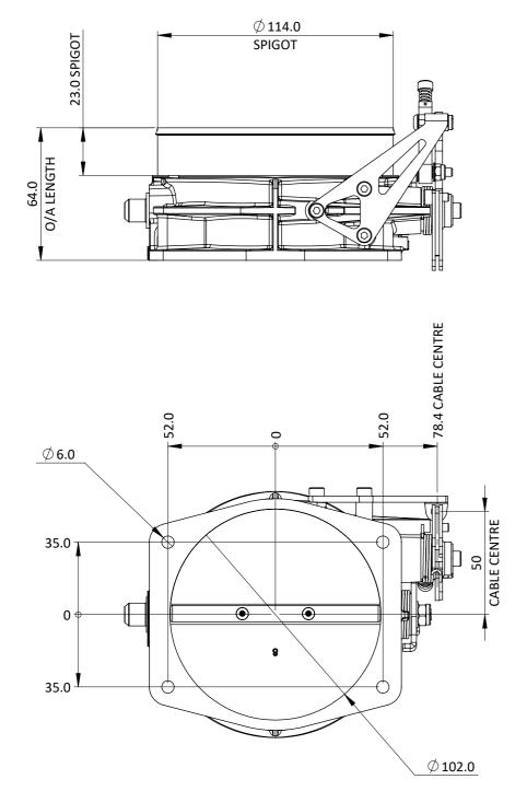
Very large single bore motorsport throttle body with 102mm bore.
