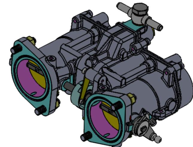
The Heritage body is designed with major dimensions identical to twin vertical carburetors from Weber, Dellorto, Solex etc. The fuel rail is integrated within the body lid, supplied with Bosch EV14 730cc/min injectors. The body comes with 'O' rings on the outlet, idle bypass adjustment, 60mm long air-horns and an internal throttle position sensor. Operating data; Spindle rotation: 82 degrees.
