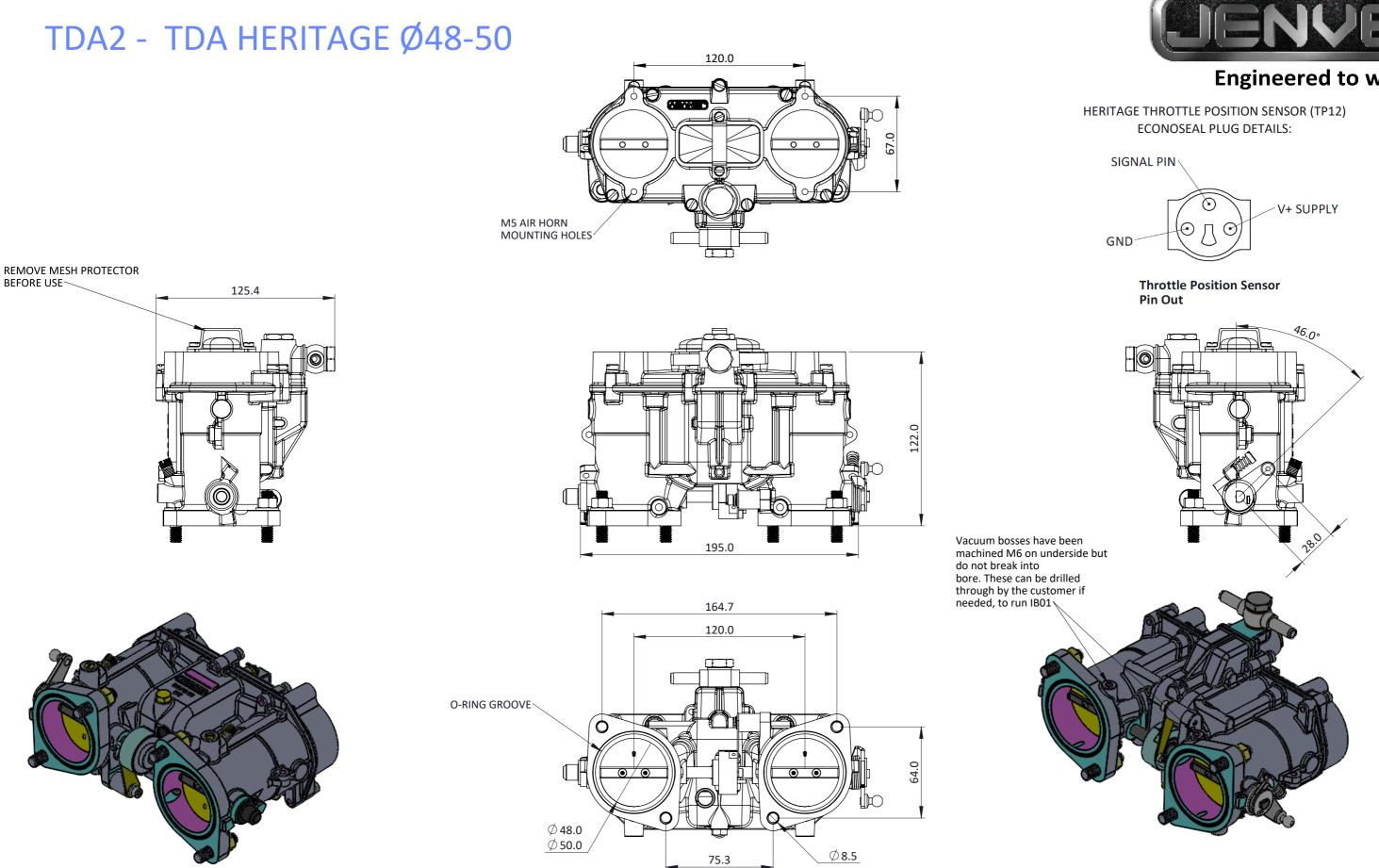
The Heritage body is designed with major dimensions identical to twin vertical carburettors from Weber, Dellorto, Solex etc. The fuel rail is integrated within the body lid, supplied with Bosch EV14 730cc/min injectors.
